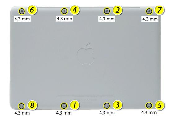
**5** Tilt up and remove bottom case.
